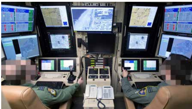
The Ground Control Station allows pilots to fly from thousands of miles distance
