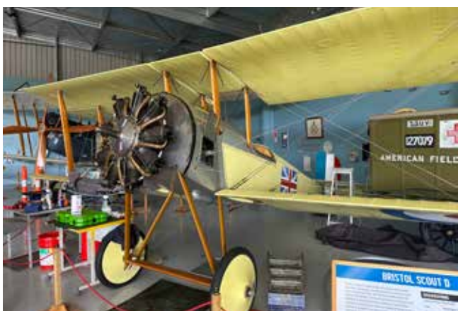
Bristol Scout with American-made Le Rhône rotary engine
